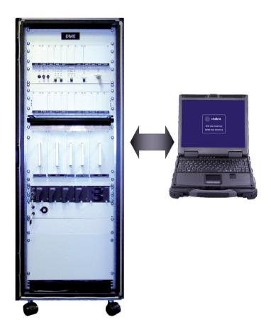
The result of Indra's expertise in radio navigation is a new distance measuring equipment highly reliable and low cost
