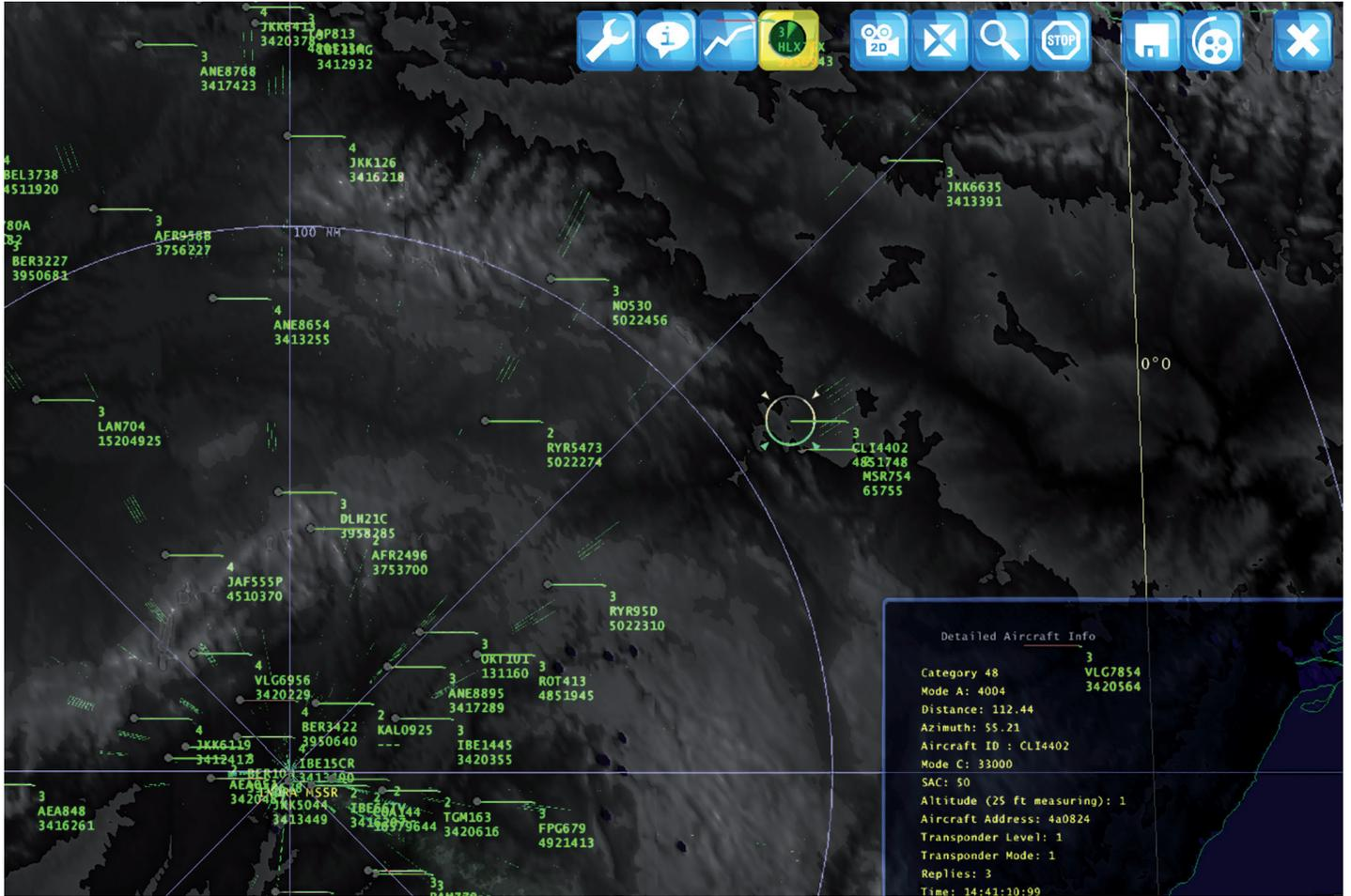
Screen from the side local central and monitory position showing mod S Asterix data and raw video in 3D view
